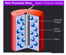
and launches the shell out the other end. The lifting charge not only launches the shell it also ignites the fuse of the firework, which burns while the shell rises to its correct altitude, where it then lights the bursting charge and the firework explodes. The explosion ignites the outside of the stars, which begin to burn with bright showers of sparks. The explosion disperses the stars in all directions, causing the light displays that we see.
